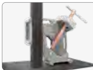
Use in upright position thanks to machined outer face.
