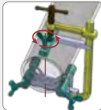
Turn three adjustment screws to preset.
